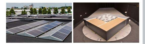
This is based on the specific wind tunnel research conducted by Peutz bv into the wind load on the Esdec FlatFix Fusion mounting system for flat roofs. This dedicated wind tunnel studies, specifically for this system, were carried out by Peutz bv in 2018 and 2023.
